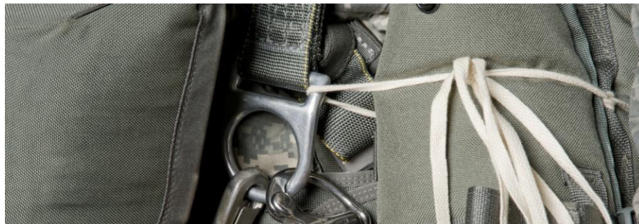
Figure 7A. Upper Tie Down Tape properly routed on the T-11 harness.
