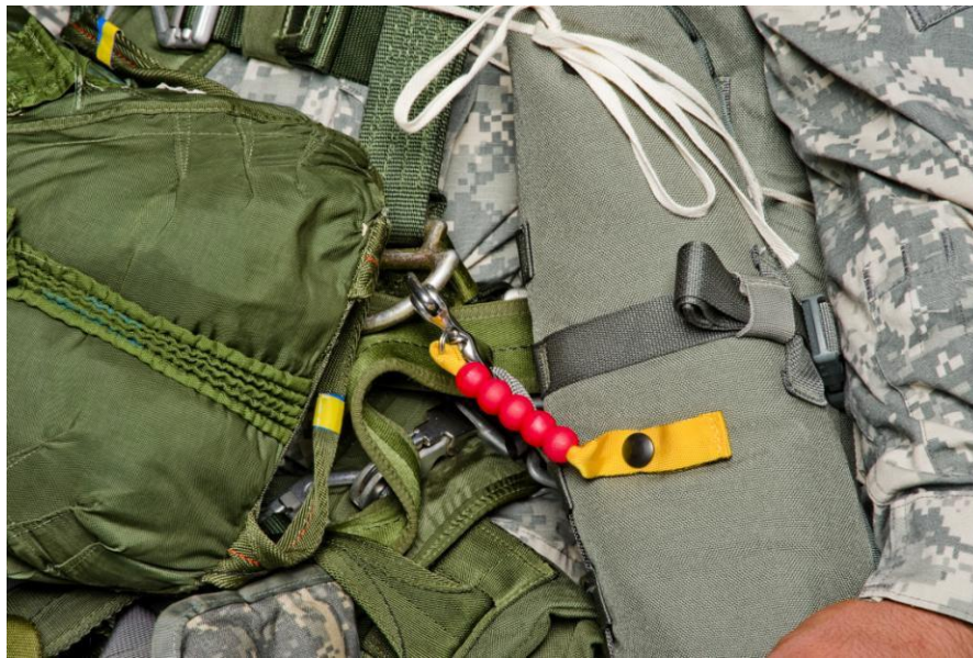
Figure 1A. Snap Shackle properly attached.
