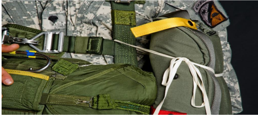
Figure 8A. Upper Tie Down Tape properly routed on the T-10 harness.
